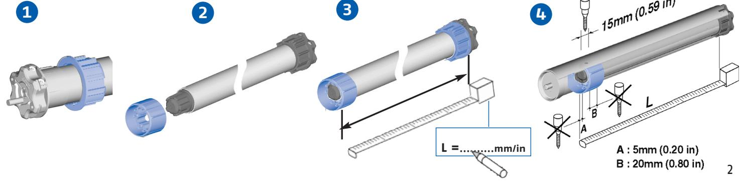
**GB** Install the tube on the brackets
